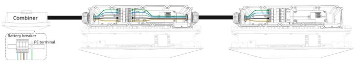
Section B. Wire the CAN communication cable
