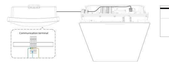
c. For the battery 1, remove the resistor on the C1 and C2 terminal, and then connect the cable to the C1 and C2 terminal as below.
