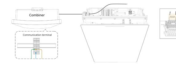
d. Connect the cable to the C1 terminal as below.
