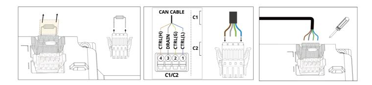
e. Arrange the cables and check the wiring is correct.
