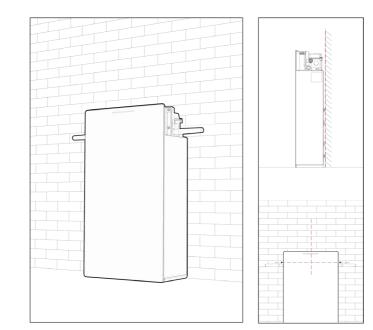
d. Remove the handlebars and take out the mounting lugs and align them with the holes on the both sides. Insert the M10 screws and tighten the screws with a torque of 9–14 N·m.
