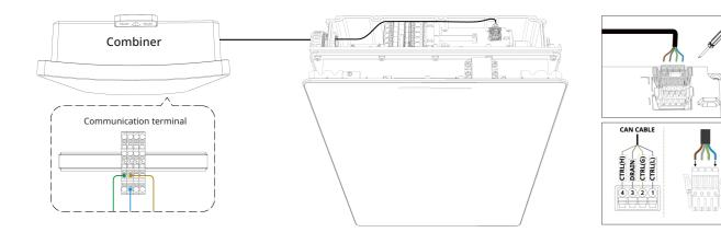
e. Arrange the cables and check the wiring is correct.
